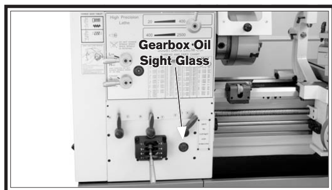
Figure 112. Gearbox sight glass location.
